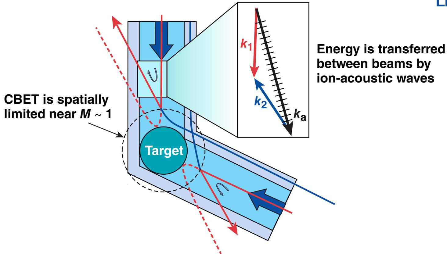
**CBET reduces the most hydrodynamically efficient portion of the incident laser beams.**
