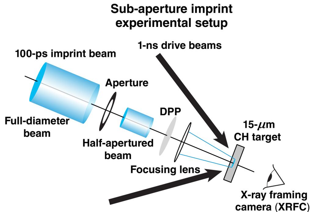
The effect of an increased imprint power spectrum resulting from the reduced beam diameters was tested in planar experiments.
