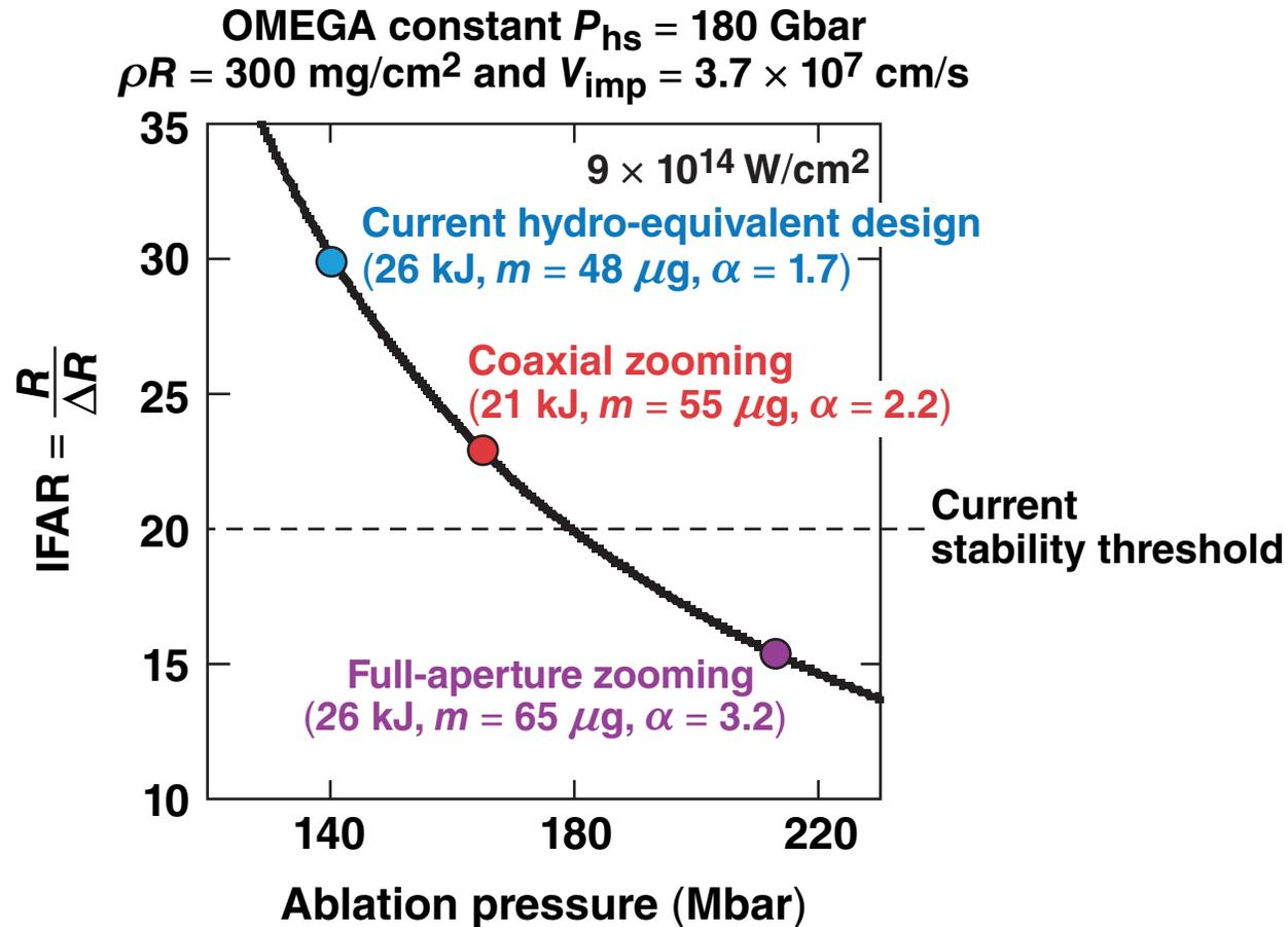
A full-aperture zooming scheme (that will maintain excellent smoothing) is being developed that uses bandwidth to control the focal-spot size.
