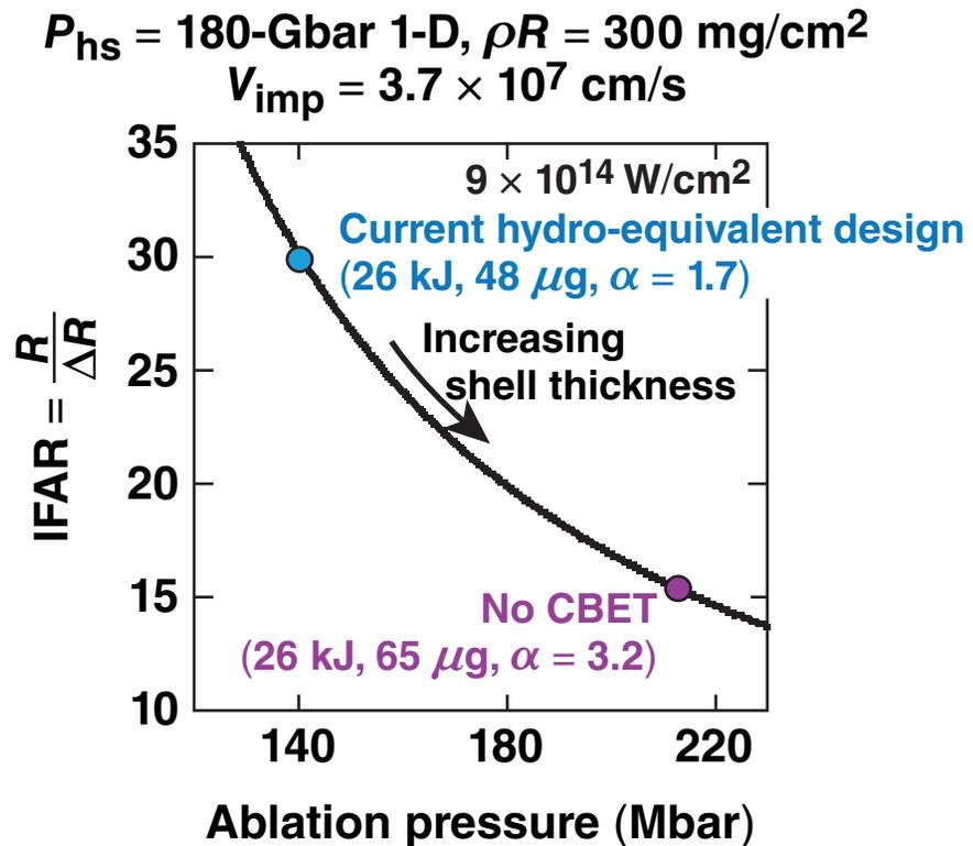
Experiments have demonstrated that CBET can be mitigated by reducing the energy that propagates past the target.
