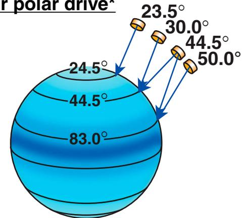
2-D simulations predict polar-drive ignition on the NIF when appropriate beam smoothing has been added.
