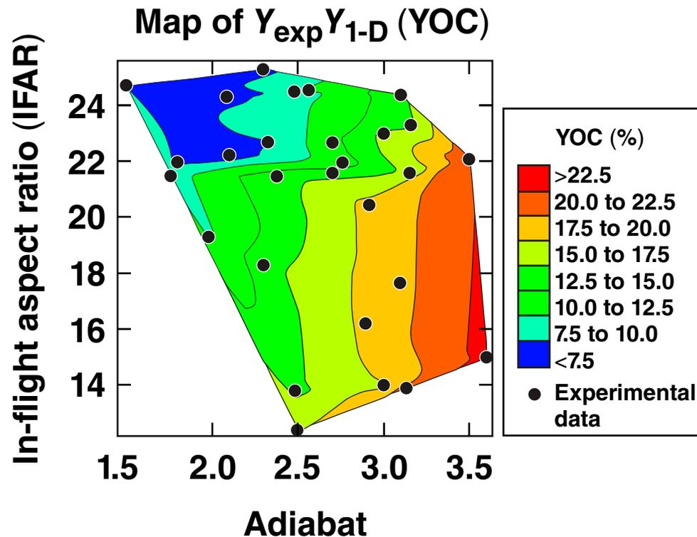
The 1-D simulations include all of the known physics with no adjustable “knobs.”
