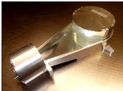
Pilot B plastic scintillator, 17.78-cm diam, 10-cm thick, Photek PMT-240 gated PMT two-stage MCP, gain  $10^6$  at 12.4 m from a target
