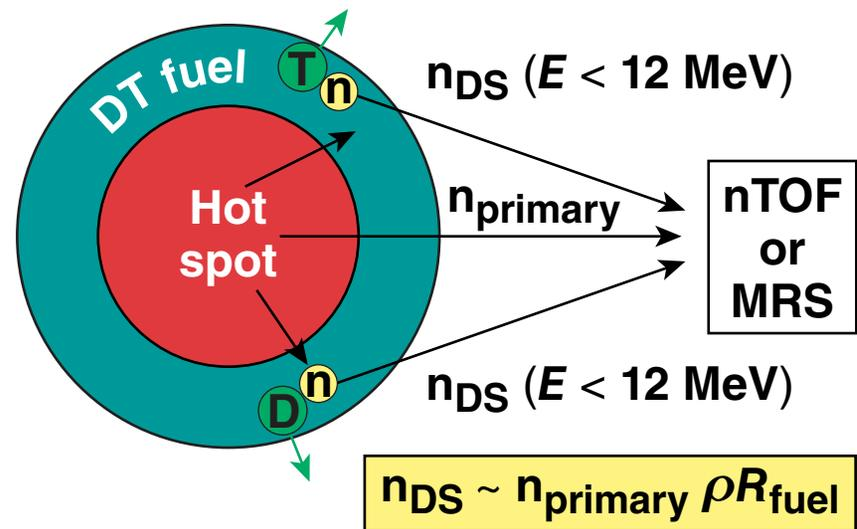
Much of our recent effort has focused on how to measure the “down-scatter fraction” using nTOF techniques—we are testing a solution now!
