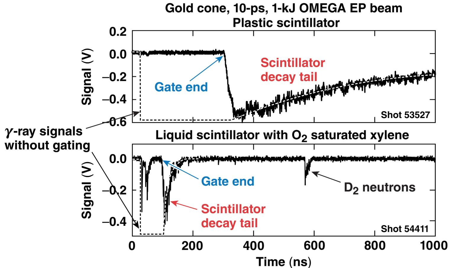
This nTOF detector was used in FI experiments to measure the D<sub>2</sub> neutron yield.
