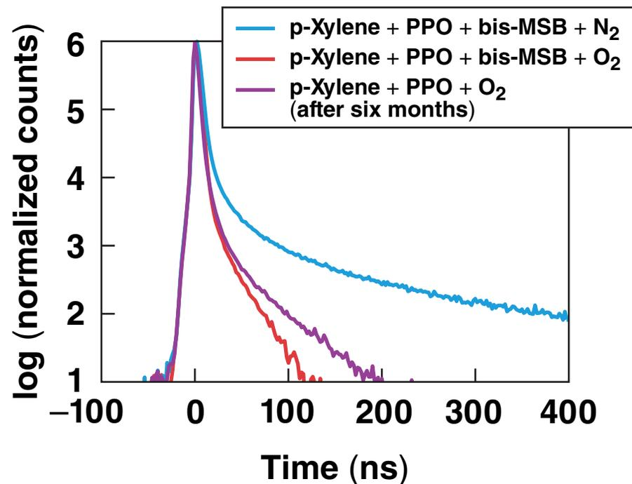
Liquid scintillators enriched with an O<sub>2</sub> quenching agent have a fast-decay time—the  $\gamma$ -ray-induced fluorescence is efficiently suppressed.
