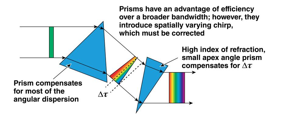
An N-KZFS2 prism (apex angle = 74°) and an SF57 prism (apex angle = 24°) reduces angular dispersion from 15 mrad to 10  $\mu$ rad and has a spatially varying chirp ( $\Delta \tau$ ) of <10 fs.
