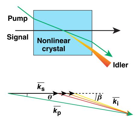
OPA is a three-wave mixing process inside a nonlinear crystal
