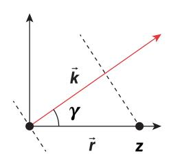
Spectral phase is proportional to the optical distance traveled by a wavefront of a plane wave between two points
