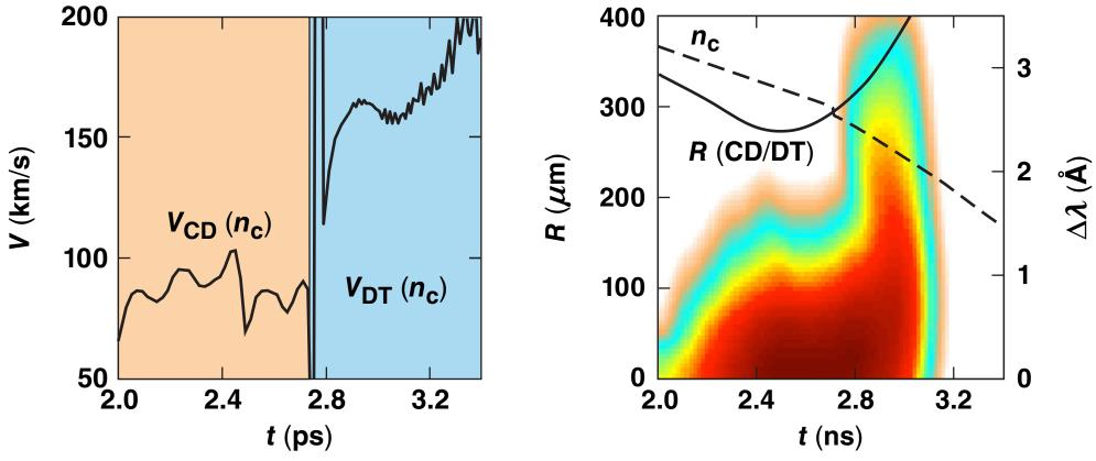
When the DT reaches the absorption region, the velocity of the critical surface jumps, resulting in a jump in the maximum red-shifted wavelength in the scattered-light spectrum.
