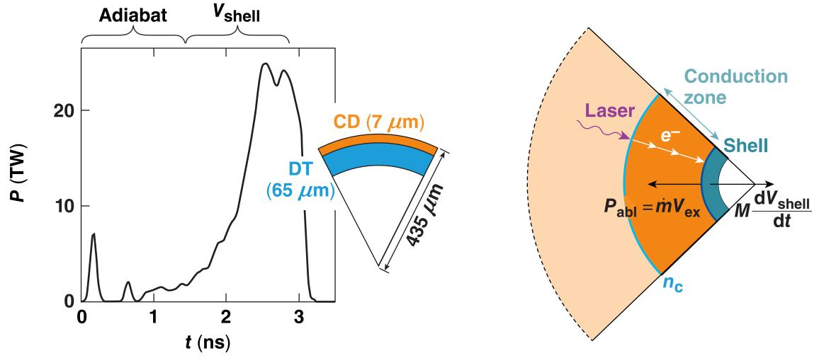
Measurement of the mass ablation rate and the size of the conduction zone constrain the hydrodynamic coupling.
