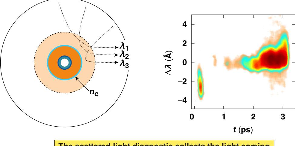
The scattered-light diagnostic collects the light coming from every beam with various angles of incidence.
