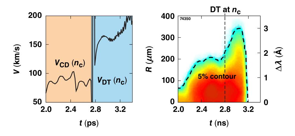
This jump in a red-shifted light provides a measure of the time when the DT reaches the absorption region.
