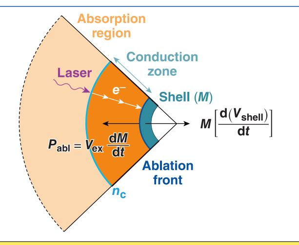
Measurements of the shell trajectory ( $V_{shell}$ ) and mass ablation rate (d*M*/dt) constrain the coupling physics.
