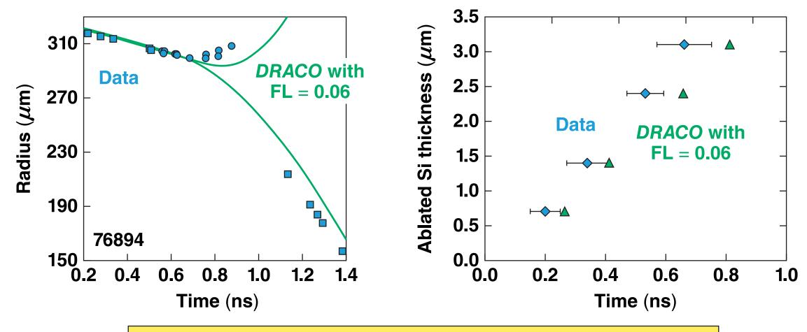
The flux-limited (FL = 0.06) model predicts a slower shell velocity and lower mass ablation rate than measured.
