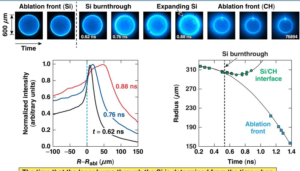
The time that the laser burns through the Si is determined from the time when the interface (outer peak) and ablation front (inner peak) separate.
