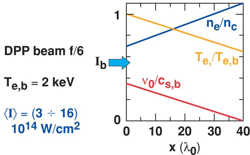
Profiles of density, flow, and temperature modeling OMEGA plasma near critical density (similar to simulations by *SAGE*).
