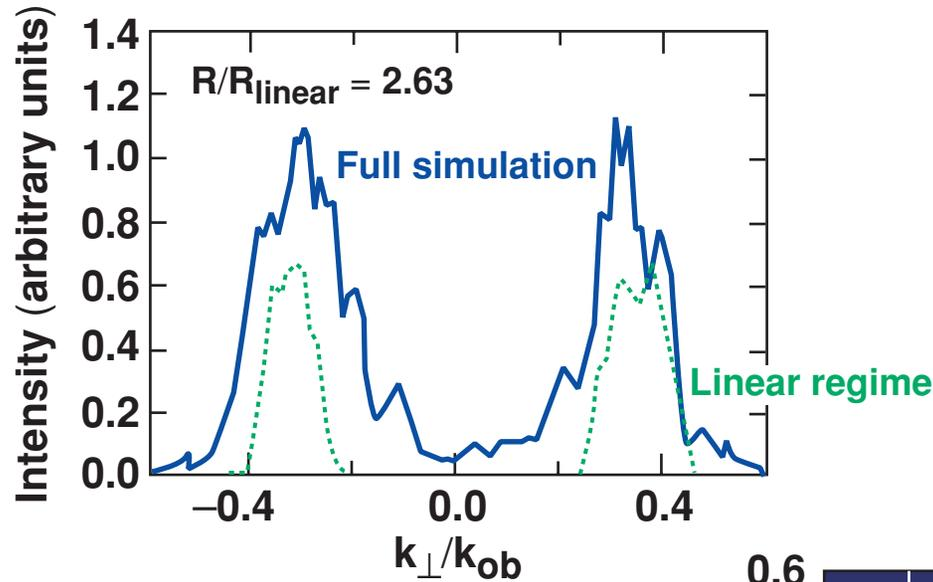
Two DPP beams with average intensity  $\langle I \rangle_{14} = 4.5$  in each beam and angle of incidence  $\pm 20^\circ$
