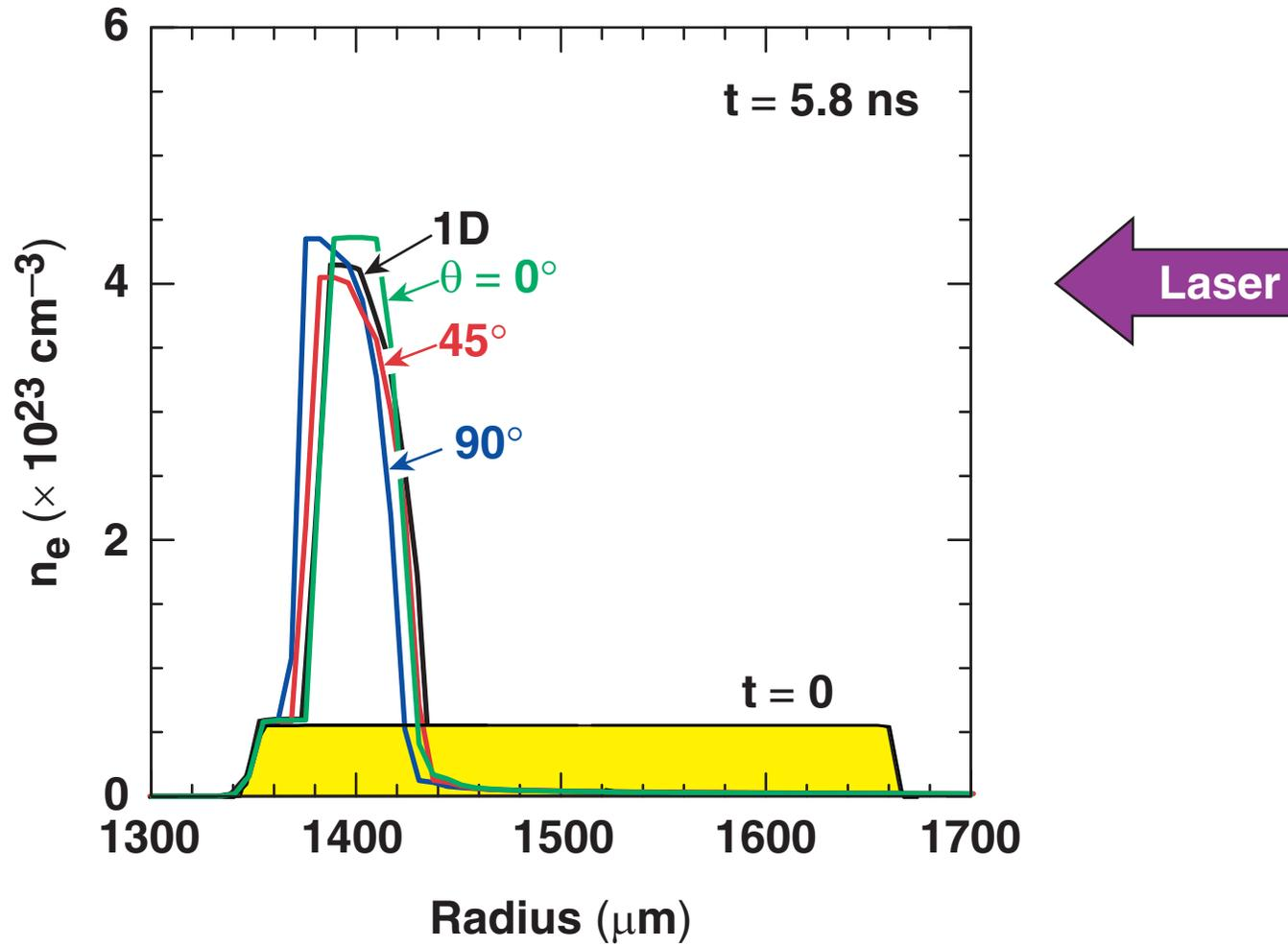
The corona is hotter and steeper at  $\theta = 90^\circ$  for the polar design
