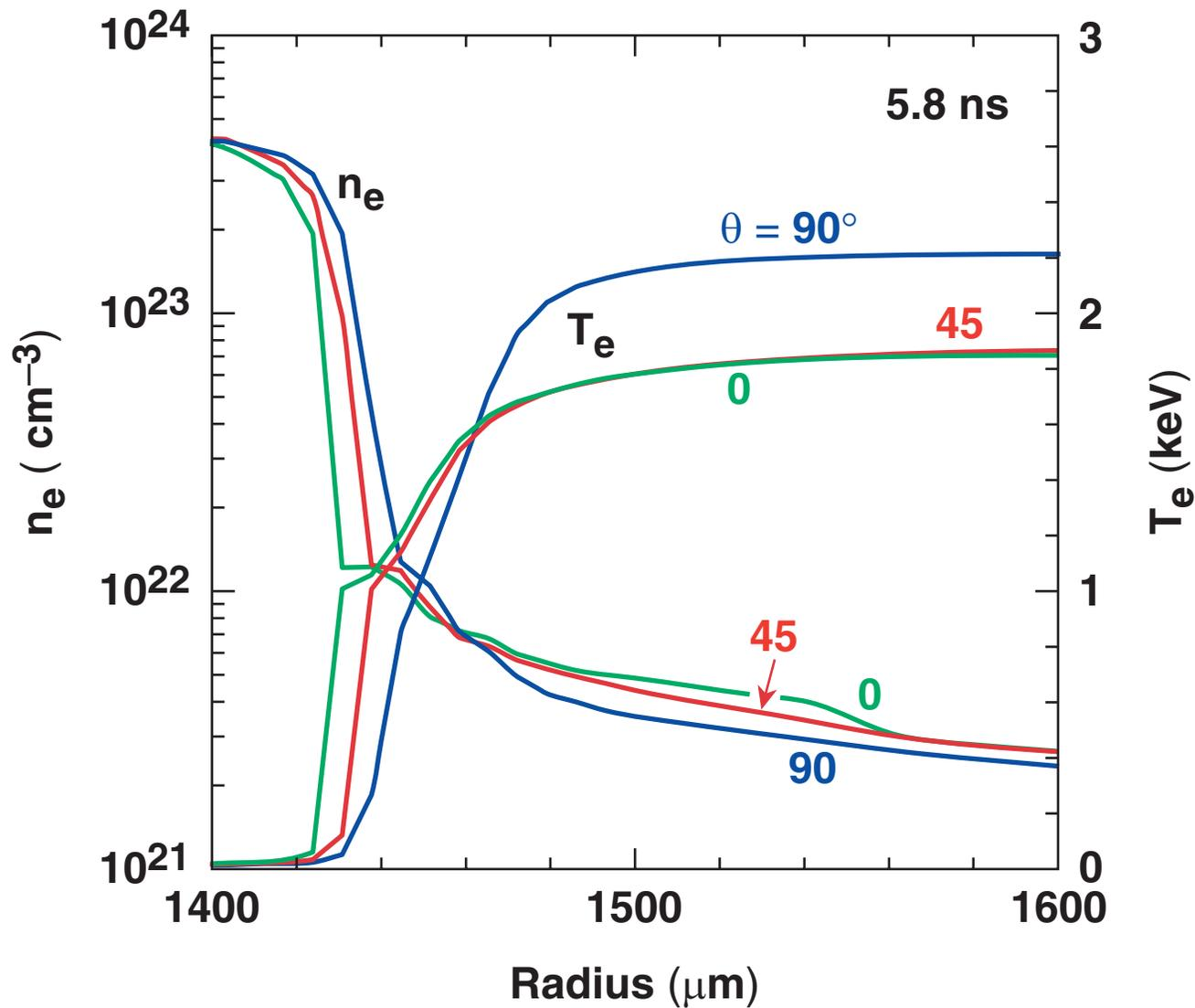
At 5.8 ns, the electron-temperature contours in the polar case show an ~10% enhancement near the equator
