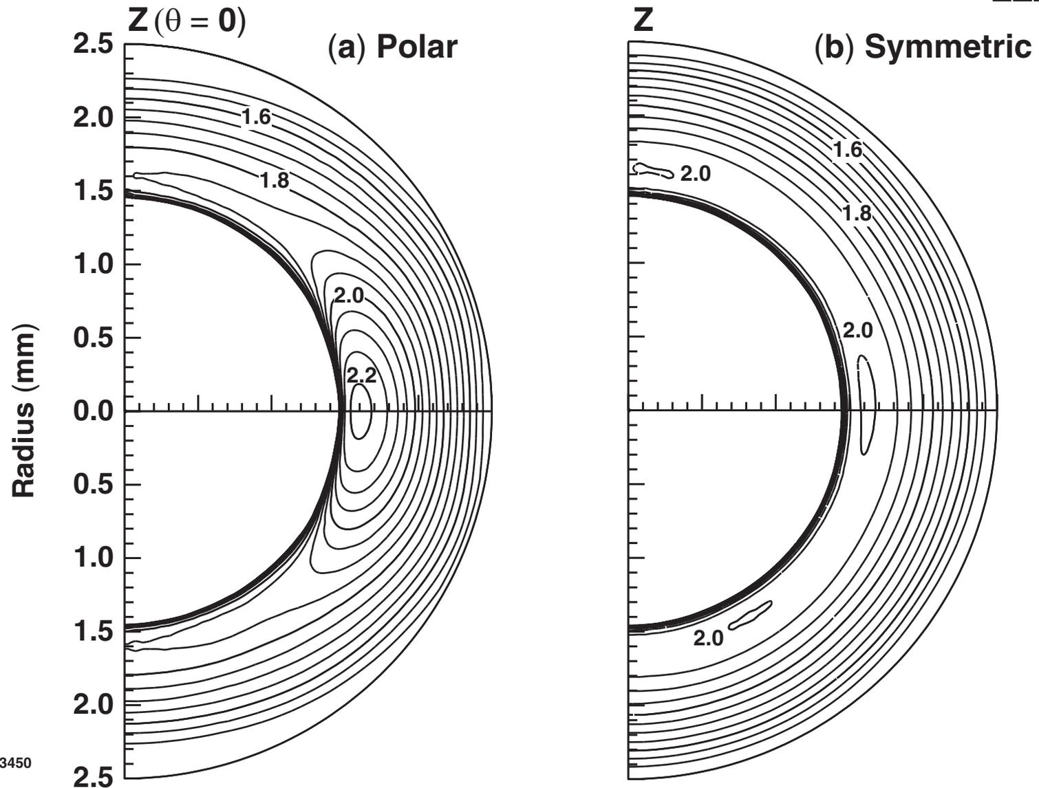
At the end of the laser pulse (9 ns), the polar case is almost as uniform as the symmetric case
