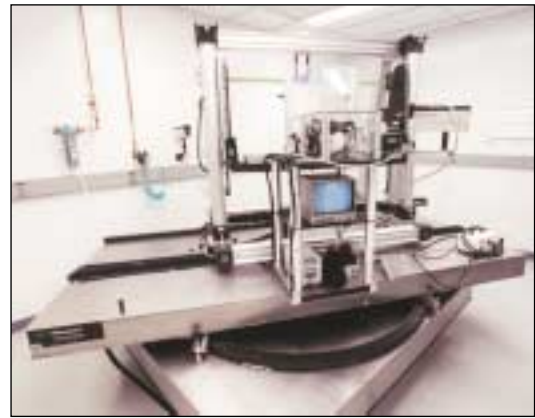
Figure 88.11 The LAC station monitors an optic’s surface quality at the same time it is being damage tested. The translation stage shown here can handle a variety of NIF optics, such as a NIF polarizer, which is 810 × 420 mm. Pictured on the stage is an LM2 substrate, approximately 420 × 420 mm.
