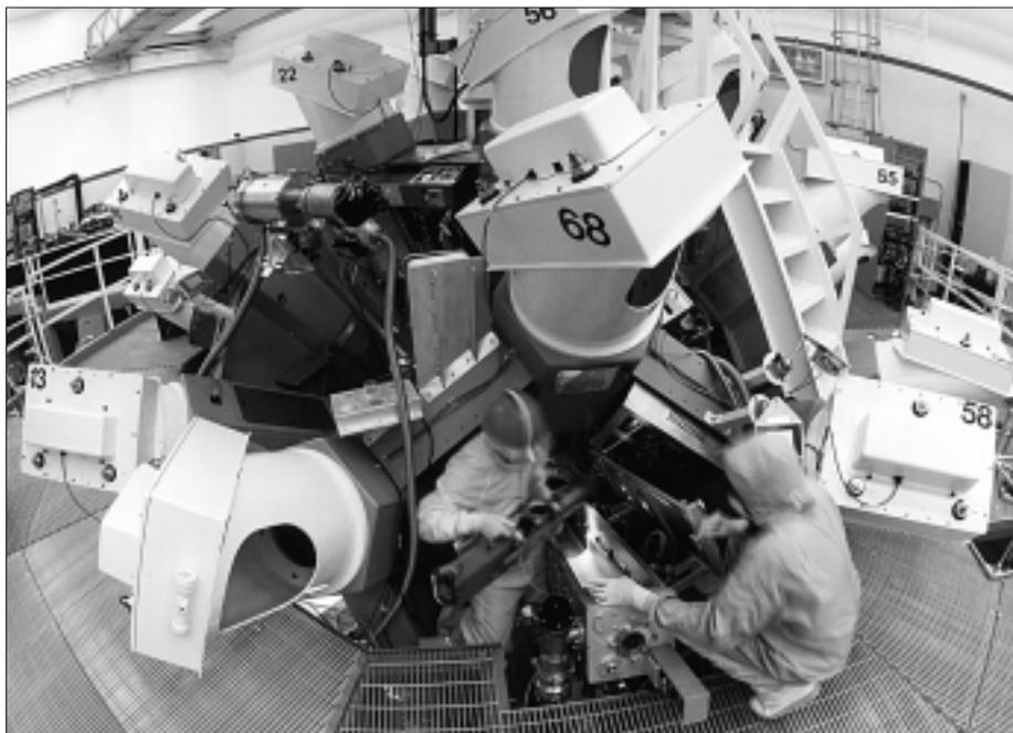
The diagnostics on the OMEGA system are divided between those that are permanently attached to the target chamber and those, such as the streak camera shown in the photograph, that are inserted with one of the six OMEGA TIM's. TIM-based diagnostics are removable and can be reconfigured between system shots. The TIM's provide a great deal of flexibility in the configuration of diagnostic systems to meet the needs of the various experiments.
