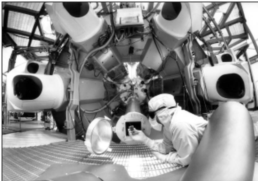
Shown at left is a wide-field view of the OMEGA target chamber's diagnostic port (H13), which contains a KB microscope with a CID camera at the image plane (the long tube pointing downward). The final beam injection mirrors surround the port. A pinhole camera with CID-camera readout is located just above the KB microscope.
