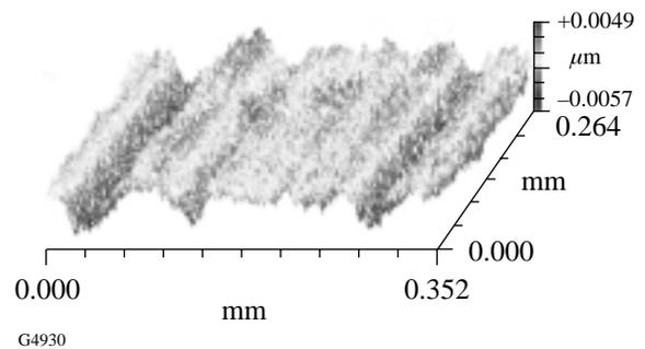
Figure 80.22 Representative optical roughness map<sup>8</sup> of the initial single-point-diamond-turned surface of KDP used for these experiments. The diamond-turning marks are clearly visible. Microroughness:  $p_v = 15.6 \pm 3.9 \text{ nm}$ ;  $rms = 1.5 \pm 0.1 \text{ nm}$ .
