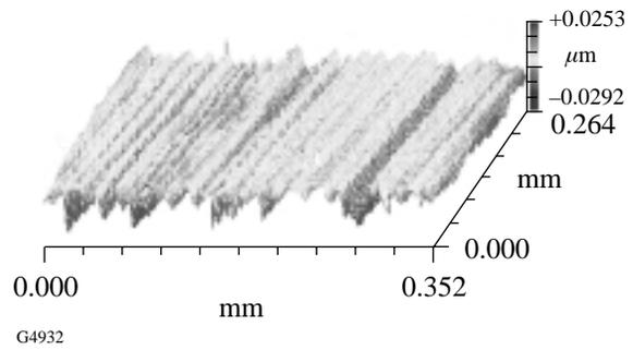
Figure 80.24 Optical roughness map<sup>8</sup> of spot made on SPDT KDP part using MR fluid without nonmagnetic abrasive. Microroughness:  $\text{pv} = 64.8 \pm 15.8 \text{ nm}$ ;  $\text{rms} = 6.4 \pm 0.8 \text{ nm}$ .
