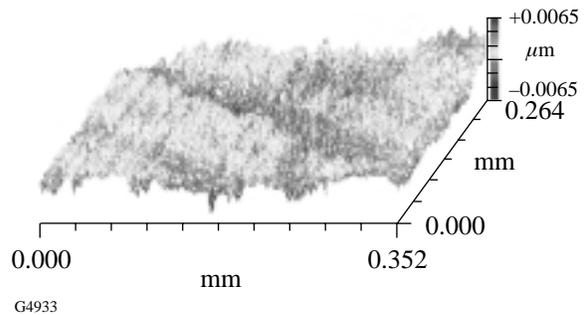
Figure 80.25 Optical roughness map<sup>8</sup> of surface within spot made on SPDT KDP part with MR fluid with 0.05-vol % nanodiamond abrasive. Microroughness:  $\text{pv} = 20.1 \pm 7.1 \text{ nm}$ ;  $\text{rms} = 1.6 \pm 0.3 \text{ nm}$ .
