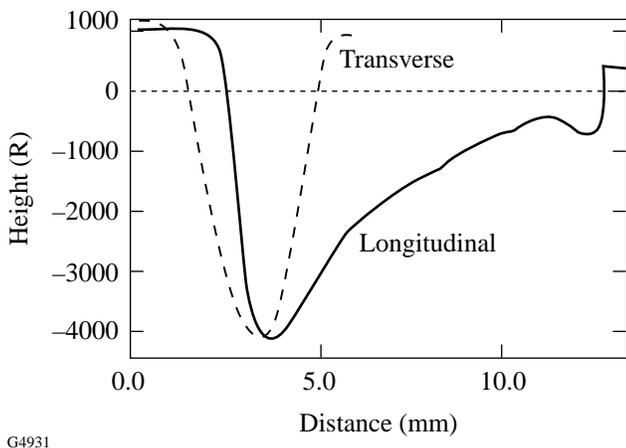
Figure 80.23 Longitudinal and transverse profile scan<sup>7</sup> of a spot made on SPDT KDP with MR fluid without nonmagnetic abrasive. Peak removal rate was  $1.59 \mu\text{m}/\text{min}$ ; depth of deepest penetration was  $0.53 \mu\text{m}$ .
