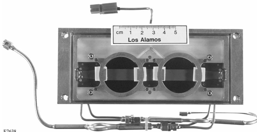
Figure 66.14 The LANL framing camera modules that are used in the GMXI.
