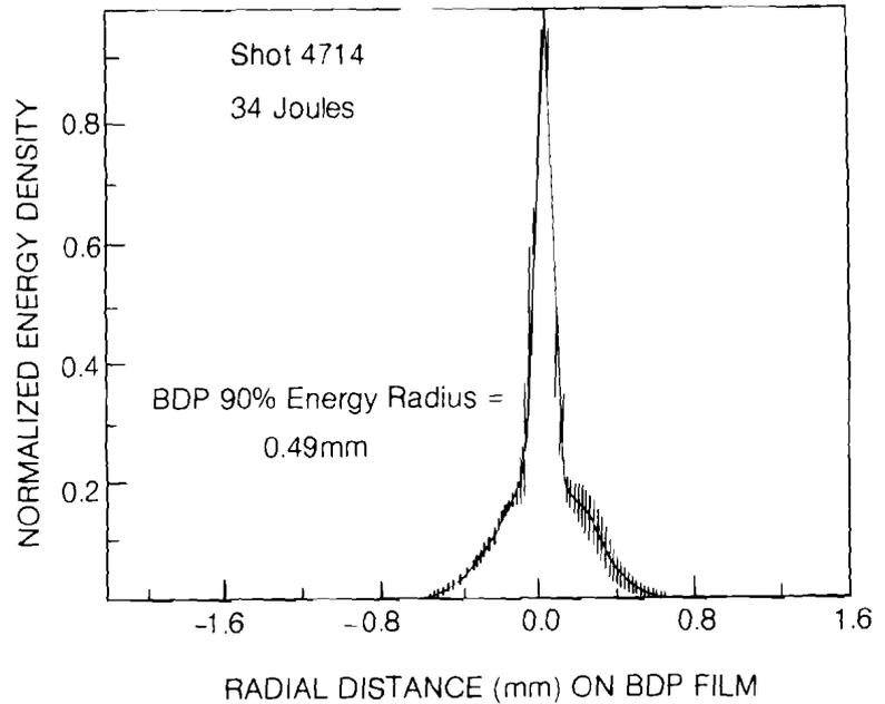
The BDP uses a 4.5 meter focal length lens to produce a photograph of the beam at the equivalent target plane on 35mm film. Experience with ZETA has shown that there is a high correlation between the BDP equivalent target plane photographs and the x-ray emission as seen in pinhole camera photographs of gold coated targets. Thus, the BDP can be used as a diagnostic to determine on-target beam quality.
