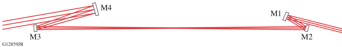
Figure 1 The final layout of the AIR mirrors, showing the ray path from the central field point.
