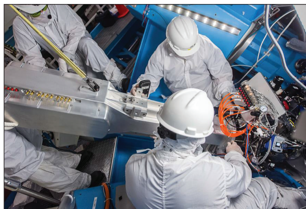
Figure 154.23 Installation of the SLOS-TRXI diagnostic on the OMEGA target chamber.
