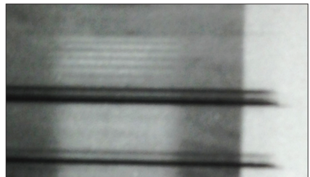
Figure 140.93 Space-resolved absorption spectrum obtained on OMEGA EP using face-on broadband spectroscopy from a Zn bremsstrahlung continuum backlighter. Photon energy increases from top to bottom; emission is dark and absorption is light. Multiple time-resolved absorption and time-integrated emission features of hot silicon are detected with an excellent signal-to-noise ratio.
