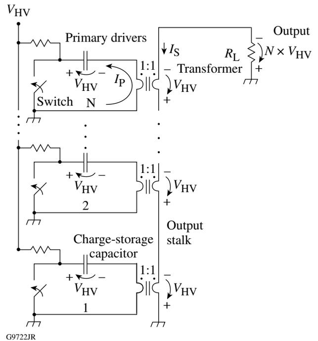
Figure 133.66 Inductive-adder schematic. When the switches simultaneously close within the  $N$  primary driver circuits, the charge-storage capacitance creates a current in the primary circuit of each coupled inductor (transformer). This current is inductively coupled to each transformer secondary and creates a voltage equal to the capacitor charge voltage. The secondary of each transformer is series connected to add the pulse voltage from each primary circuit and apply it to the load  $R_L$ .
