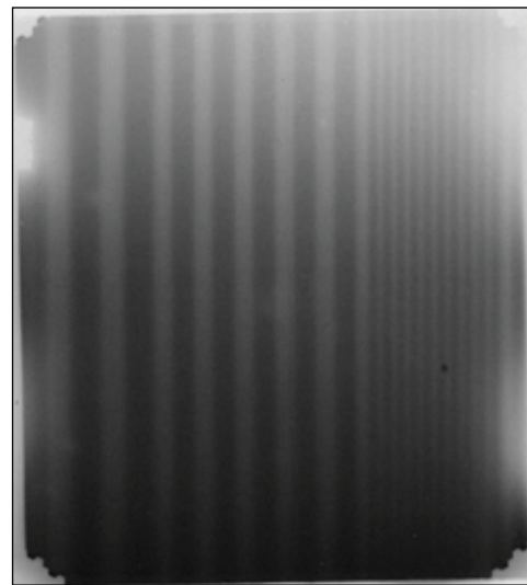
Figure 128.92 Radiograph collected on a single-strip XRFC of a Au grid backlit using a 5- \mu m-thick Ag microflag.
