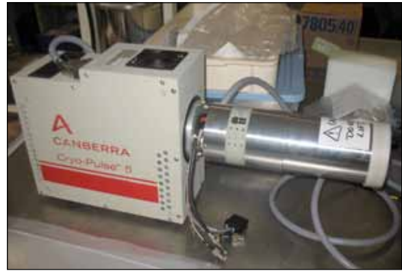
U1031JR Figure 120.119 Germanium detector with its electronic cryogenic module.
