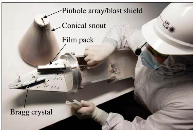
LLE experimental operations technician Ben Ruth adjusts the film pack of the x-ray spectrometer (XRS), which is shown with the conical snout removed. X rays from the target propagate through the blast shield and pinhole array, diffract from the Bragg crystal, and are detected on film.
