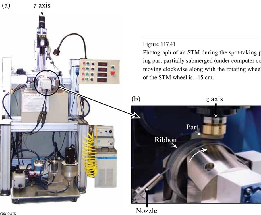
Figure 117.41 Photograph of an STM during the spot-taking process: (a) spot-taking machine; (b) the nonrotating part partially submerged (under computer control) into the stiffened MR fluid ribbon, which is moving clockwise along with the rotating wheel. The STM has only  $z$ -axis motion. The diameter of the STM wheel is  $\sim 15 \text{ cm}$ .
