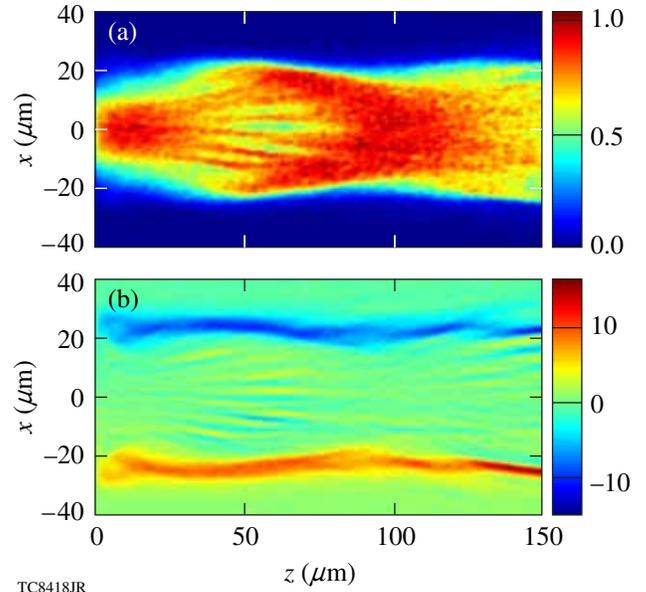
Figure 117.32 (a) Hot-electron density (in  $\text{cm}^{-3} \times 10^{21}$ ) and (b) magnetic field (in MG) 700 fs after the peak of the laser pulse in the simulation for a compressed uniform plastic target and a laser pulse with a focal-spot diameter of  $20 \mu\text{m}$  and a maximum intensity of  $6 \times 10^{19} \text{ W/cm}^2$ .
