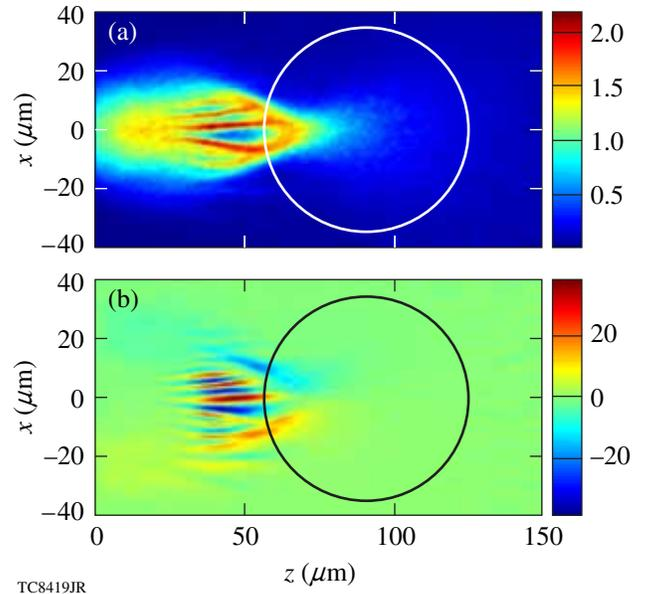
Figure 117.33 (a) Hot-electron density (in  $\text{cm}^{-3} \times 10^{21}$ ) and (b) magnetic field (in MG) 700 fs after the peak of the laser pulse in the simulation for a compressed plastic target with a Gaussian spatial density distribution, and a laser pulse with a focal-spot diameter of  $20 \mu\text{m}$  and a maximum intensity of  $6 \times 10^{19} \text{ W/cm}^2$ .
