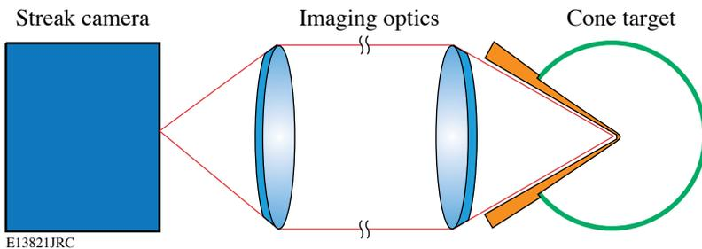
Figure 103.10 Streaked optical pyrometry (SOP) setup used to investigate the filling of the inside of the cone.
