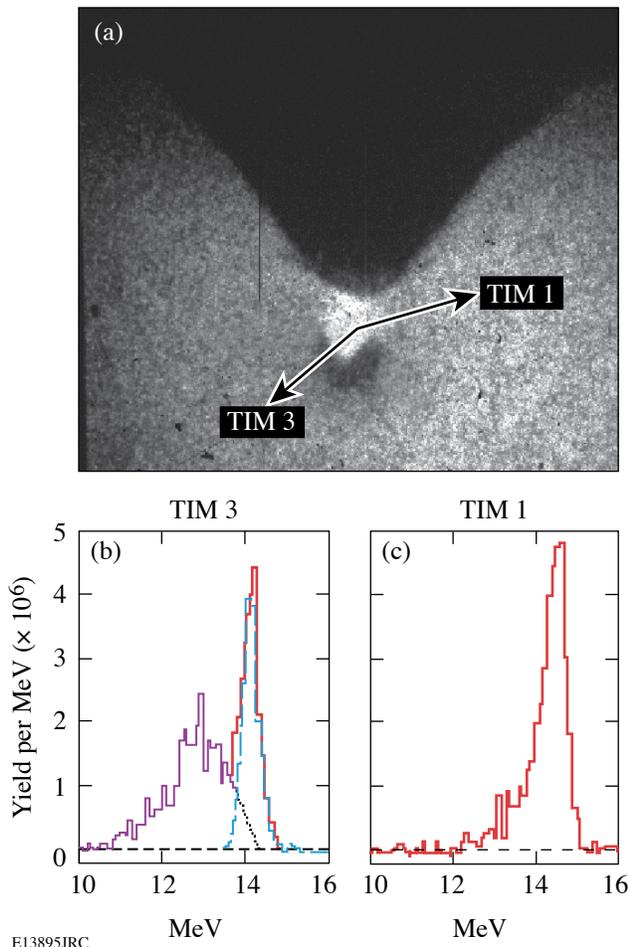
Figure 103.9 Backlit image (a) of a 10-atm,  $D^3He$ -filled cone target at time of peak proton production using a Fe backlighter. Significant self-emission from the hot  $D^3He$  gas is seen in the image. The directions of the proton spectrometers used to determine the core areal density are indicated as TIM1 and TIM3.  $D^3He$  proton spectra taken along two different lines of sight: TIM3 (b) and TIM1 (c).
