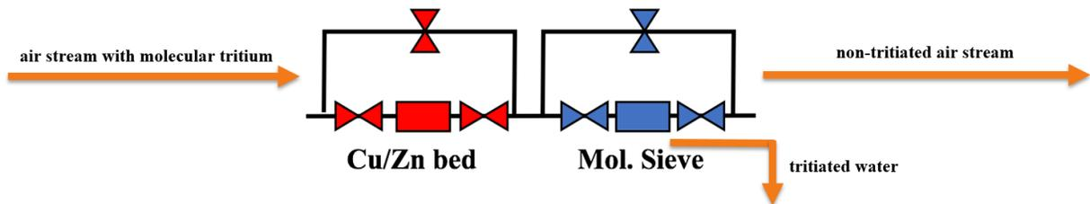
In this experiment, a Cu/Zn alloy was characterized as an alternative to replace Cu. Specifically, this experiment investigated the oxygen gettering efficiency (defined as the bed's efficiency of adsorbing oxygen) and capacity (the percentage of copper that is oxidized) as a function of bed temperature during the oxygen regeneration process and the bed's conversion efficiency of hydrogen to water as a function of oxygen inventory during the hydrogen oxidation process.
