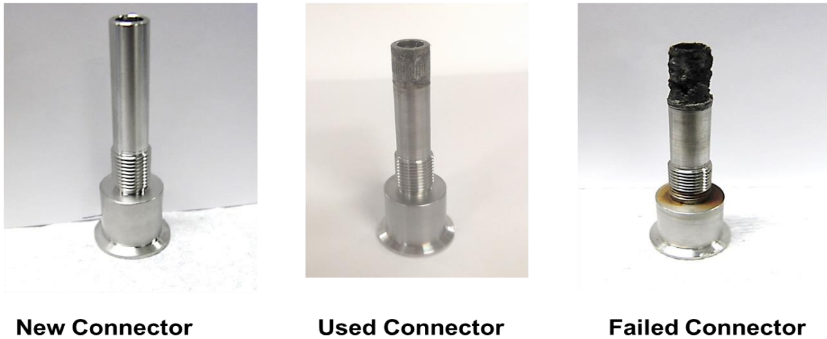
Figure 2: Progression of flash-lamp connectors from new, used, to failed.
