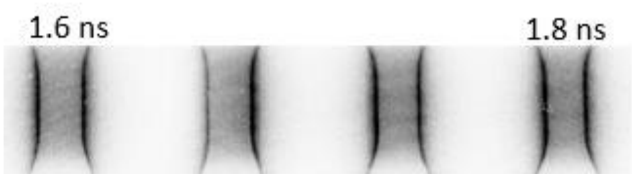
Figure 4: X-ray emission images 6 of implosion from experimental shot 79495 from 1.6 to 1.8 ns.
