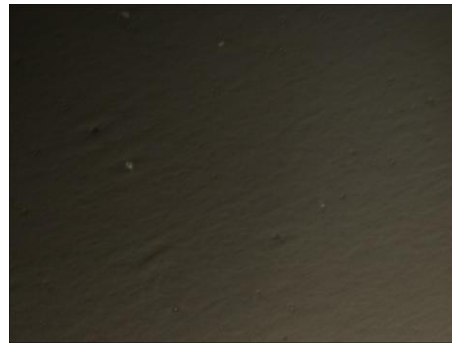
Figure 4d: A microscopic view between crossed polarizers showing the texture of the coating. There are few features and the texture is mostly smooth, which shows good coating quality.
