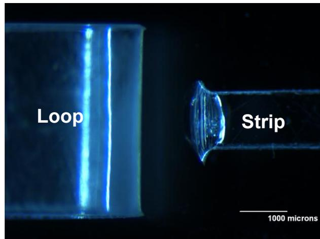
*Figure 5: Microscope view of sample after load was applied. The “golf-tee” formation is evident, as the adhesive on the strip made a clean break from the loop.*
