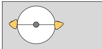
*Figure 1: Original sample preparation method. a.) The attachment of the silicon carbide fibers with Norland 68 adhesive to the polystyrene ball is viewed under a Leica microscope. b.) The attached fibers to the polystyrene were glued onto a hole-punched sheet of paper, which was then used to test the strength of the polystyrene to the adhesive in the DMA 8000.*
