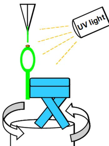
*Figure 6: Possible rotating curing system. The entire sample preparation setup would be placed on a rotating stand, as illustrated. A rotating curing system would ensure that the adhesive would be cured in a standardized, consistent method.*
