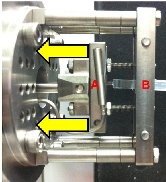
*Figure 3: Sample loaded into DMA for testing. Clamp “A” applies the increasing load to the strip, while Clamp “B” holds the loop end of the sample. The force required to break the sample is then measured.*
