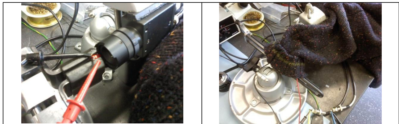
Fig. 12 Synchronous camera test setup: Red LED, left image center, pulsed on T-0 to simulate the OMEGA laser. LED points directly into camera, synchronized by V-Sync and H-Sync. Setup is isolated from room light to create contrast with LED light.
