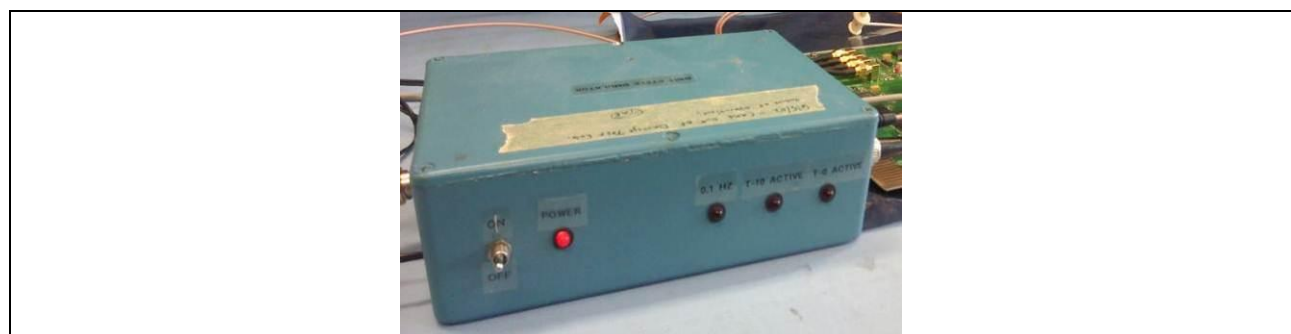
Fig. 10 Shot Cycle Simulator: Creates T-10 and T-0 enable pulses to imitate shot cycle progression. Connected to inputs of the RRM.
