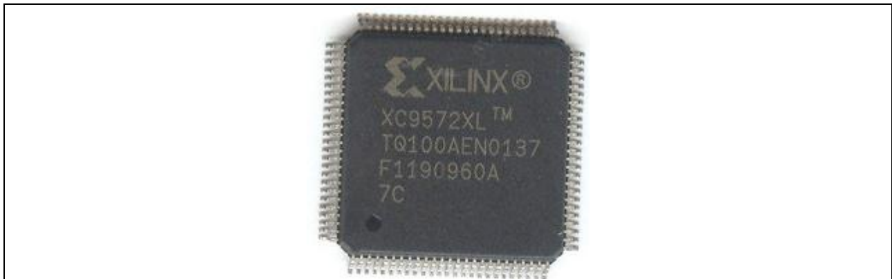
Fig. 4 CPLD: Made by Xilinx, this CoolRunner-II CPLD consumes very little power, has a very low pin-to-pin delay, and measures only 20 mm x 20 mm.
