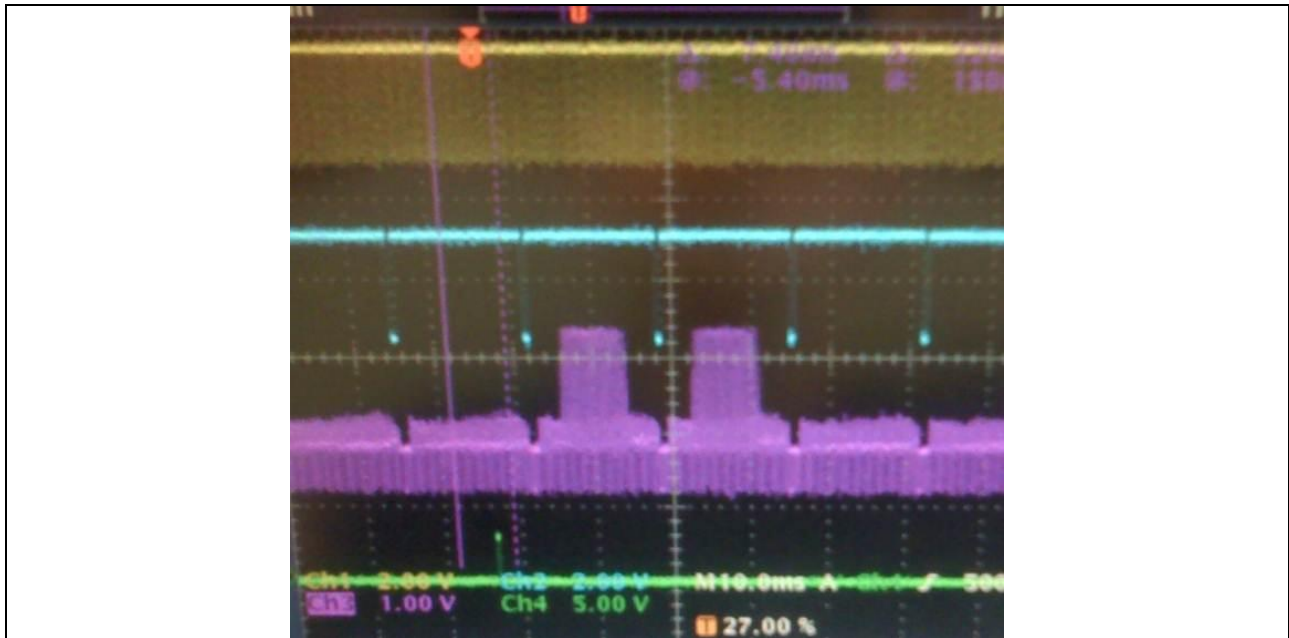
Fig. 13 Oscilloscope trace of synchronous camera test: Signals from top: H-Sync, yellow; V-Sync, blue; camera output, purple; T-0, green. The short LED pulse is shown in green near the bottom left. Since the camera uses interlaced video mode, each frame is represented by two V-Sync pulses. The next frame after the LED pulse shows spike in camera signal, or light intensity.
