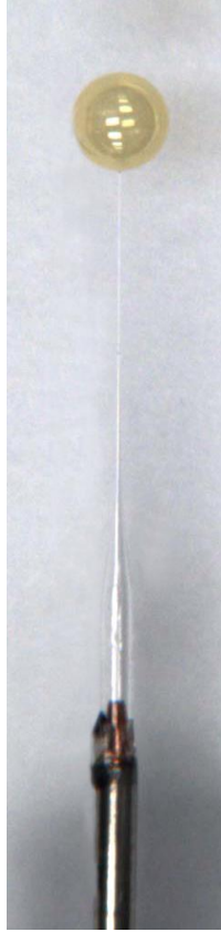
Figure 1. Photograph of a cryogenic fill-tube target with a 3 mm diameter. The fill tube enters the target with a 30 \mu\text{m} diameter.
