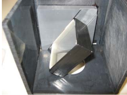
Figure 3: apparatus used to hold Brewster's angle polarizer
