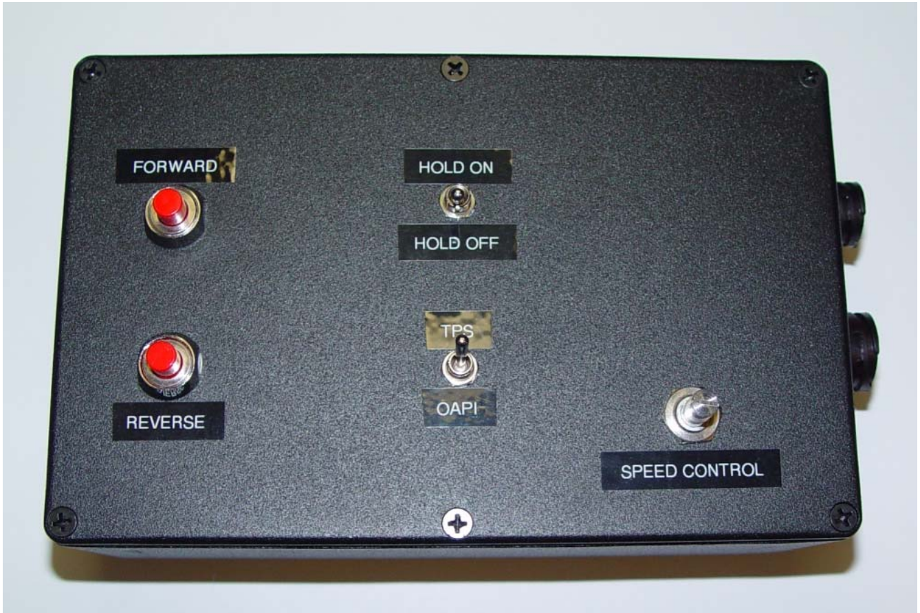
Figure 4: Photograph of the finalized test fixture. The CPC connectors on the right side provide connections to a power source and the motor, as well as the limit switches.
