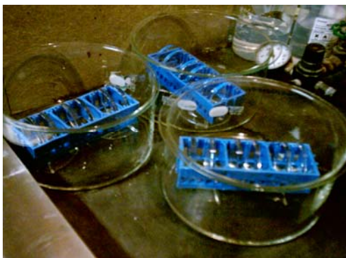
Fig. 6: General silanization setup used for all experiments. The substrates are held in Teflon racks and placed into the large glass chambers for silanization. The reactive silane is placed in the chamber and the chamber is covered. For elevated temperature studies, the chambers were placed on a digital hotplate (not shown).
