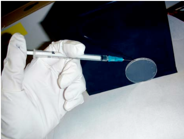
Figure 8. A vertical fill technique used to fill a cell with liquid crystals.
