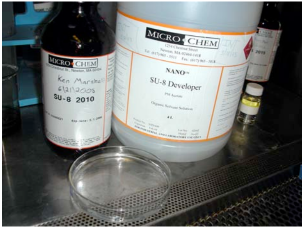
Figure 5. Immersion development process using SU-8 Developer to remove unexposed resist.
