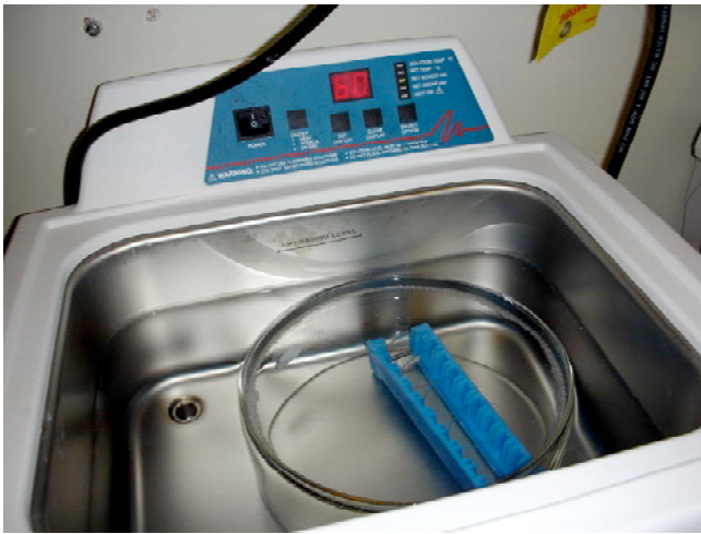
Figure 2. Cleaning of substrates in an ultrasonic bath.
