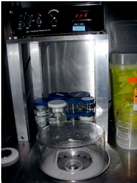
Figure 6. Spin-deposition of ROLIC photoalignment coating. The spin coater is covered with a glass dome to prevent rapid evaporation of the solvent during the deposition process.
