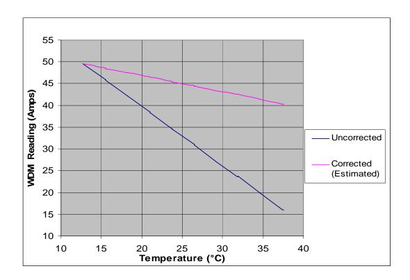
Figure 3: This graph shows the WDM's DC offset at different temperatures. The pink line shows the WDM corrected with an average correction factor. The average correction factor is not perfect due to variations between boards. Similarly, the signal sensitivity of the WDM when it is driven with sine waves (based on peak amplitude), is a linear result, with a slope of about -1.5 amps per degree Celsius (see figure 4).
