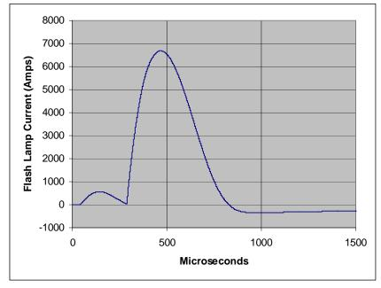
Figure 1: A typical measurement illustrating the current waveform provided to the flash lamps.
