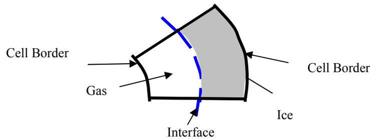
Figure 6: Cell containing the gas/ice interface. Both ice and gas are present in the cell.
