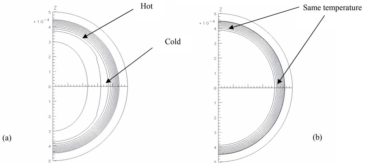
Figure 7: (a) Temperature contours in the target near the beginning of the layering process ( $t=5$  s). The presence of the ring noticeably affects the contours near the equator. The distorted contour shows that the ice surface near the equator is colder than the surface near the poles. (b) Contours after the layering ( $t=1$  h). The z axis is vertical and the outer radius is  $500 \text{ }\mu\text{m}$ . The outer radius of the target itself is  $450 \text{ }\mu\text{m}$ .
