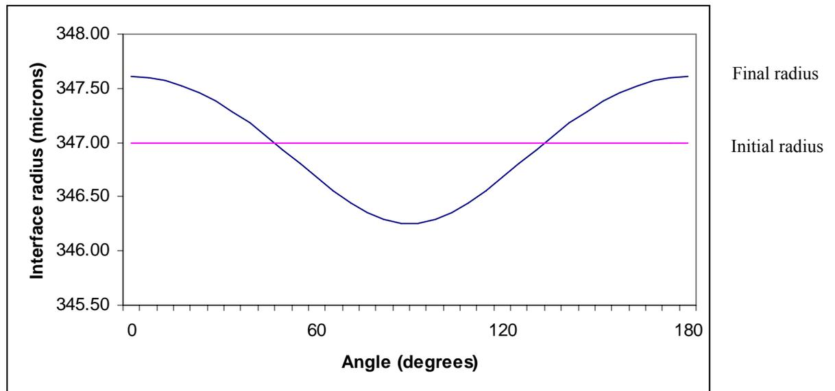
Figure 9: Ice-gas interface radius for different angles  $\theta$ . The red and blue lines represent the initial and the final radii, respectively. The initial radius was set to be uniform as a function of  $\theta$ . After layering, the ice becomes slightly thicker (the interface radius slightly smaller) near the equator ( $\theta = 90^\circ$ ) and slightly thinner at the poles ( $\theta = 0^\circ$  and  $\theta = 180^\circ$ ).
