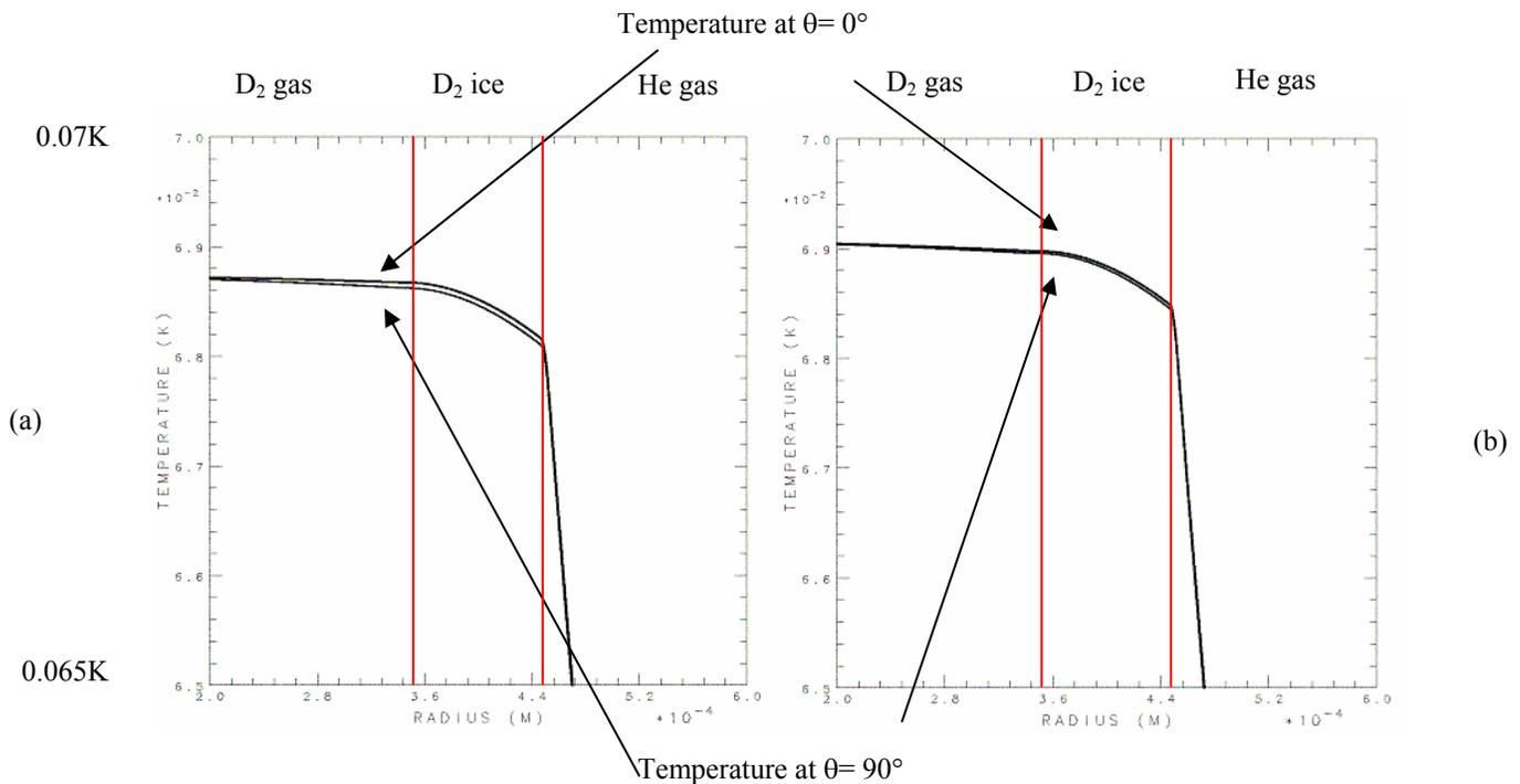
Figure 8: (a) Temperature profile as a function of radius from  $200 \mu\text{m}$  to  $600 \mu\text{m}$  near the beginning of the layering process ( $t=5$  s). (b) Temperature profile after layering ( $t=1$  h). The temperatures on the scale represent the temperature above the reference temperature of  $18.6$  K. The vertical red lines indicate the ice layer (from  $347 \mu\text{m}$  to  $447 \mu\text{m}$ ).
