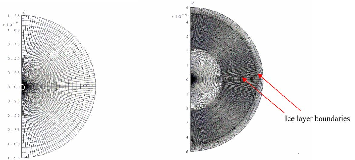
Figure 5: (a) The entire layering sphere divided into grid cells (outer radius=1.25 cm), and (b) the area outlined in white in greater detail (radius = 500  $\mu\text{m}$ ). Note the high density of grid cells in and near the ice layer, whose boundaries are shown with dark lines.
