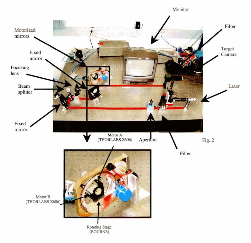
Figure 2. Experimental Setup
