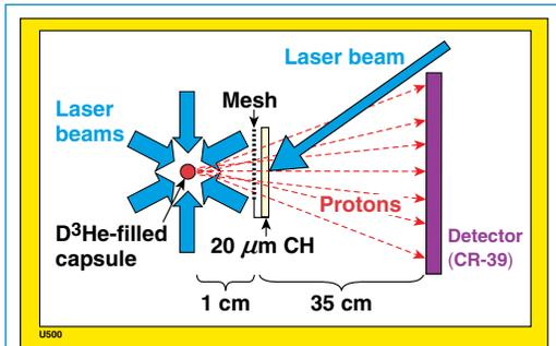
Figure 1. Physical arrangement of the proton backlighter (imploded  $D^3He$ -filled capsule), mesh, CH foil, CR-39 imaging detector, and OMEGA laser beams, as used for radiography.
