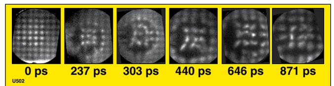
Figure 2. Images recorded on the CR-39 detectors during different OMEGA shots. Each image is labeled by the difference between the time at which the protons passed the foil and the time when the foil was struck by a laser beam. The first three images were made using a mesh with  $150\text{-}\mu\text{m}$  (center-to-center) spacing, while the last three were made with a  $200\text{-}\mu\text{m}$  mesh.
