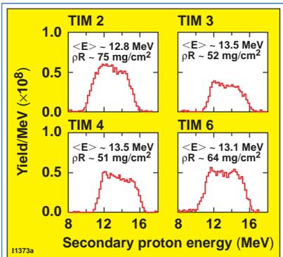
Figure 2. Secondary proton spectra from shot 28900 taken with the wedged-range-filter spectrometers (fielded in collaboration with the MIT Plasma Science and Fusion Center). The proton slowing down is consistent with a total capsule areal density of ~61 mg/cm<sup>2</sup>.
