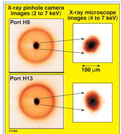
Figure 1. Time-integrated x-ray images from shot 28900 taken along nearly orthogonal directions were used to assess the implosion symmetry and placement precision of the cryogenic capsules. The target for shot 28900 was placed within 17±7 μm of the center of the target chamber.
