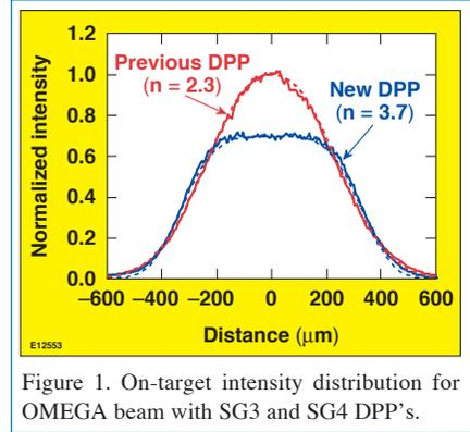
Figure 1. On-target intensity distribution for OMEGA beam with SG3 and SG4 DPP's.
