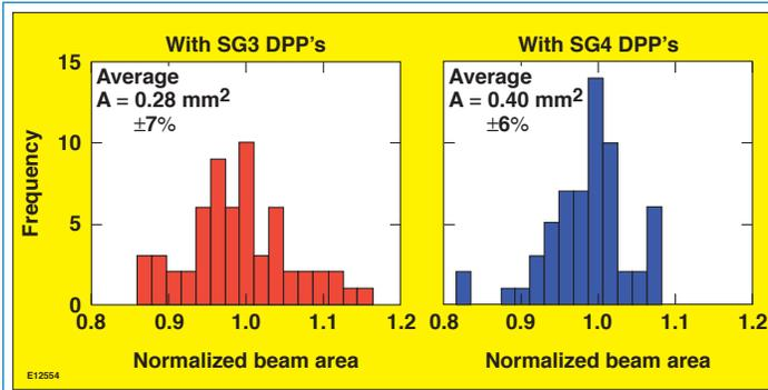
Figure 2. Comparison of the beam-to-beam size variation with the old SG3 and new (SG4) DPP's.
