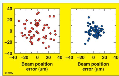
Figure 3. Pointing location of beam centers relative to ideal location as derived from eight x-ray images on OMEGA: (a) before correction, the pointing error is  $\pm 23 \mu\text{m}$  rms; (b) after repointing, the pointing error is reduced to  $\pm 11 \mu\text{m}$  rms.
