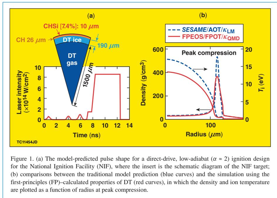
Figure 1. (a) The model-predicted pulse shape for a direct-drive, low-adiabat ( $\alpha \approx 2$ ) ignition design for the National Ignition Facility (NIF), where the insert is the schematic diagram of the NIF target; (b) comparisons between the traditional model prediction (blue curves) and the simulation using the first-principles (FP)-calculated properties of DT (red curves), in which the density and ion temperature are plotted as a function of radius at peak compression.
