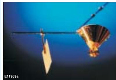
Figure 1. Photograph of a direct-drive cone-in-shell target used in recent OMEGA experiments. The target consists of an unfilled CH shell with an attached Au-coated cone. The attached foil is used for x-ray backlighting.
