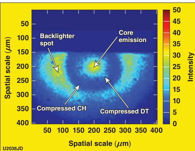
Figure 2. Radiograph of a cryogenic implosion recorded with the aberration-corrected narrowband crystal imager on a 40-ps exposure time framing camera at a convergence ratio CR  $\sim 7$ . The Si backscatterer target was driven by a 20-ps, 1.5-kJ pulse from OMEGA EP. The image is rendered on a linear intensity scale.
