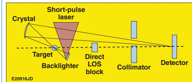
Figure 1. Schematic of the spherical crystal imager backlighting setup (not to scale). The short-pulse laser illuminates a backscatterer foil behind the primary target, which is illuminated by 60 beams from the OMEGA laser (not shown). A direct line-of-sight (LOS) block and a collimator protect the detector from background x rays emitted by the backscatterer and primary targets.
