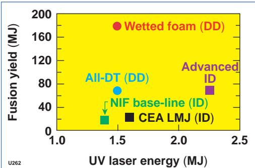
Figure 1. The calculated performance of the NIF direct-drive “wetted-foam” target (red dot) compared to several other ignition designs. The square points are for indirect-drive (ID) targets including the NIF base-line,<sup>2</sup> CEA LMJ design,<sup>3</sup> and an advanced ID design at 2.25-MJ drive.<sup>4</sup> The blue dot corresponds to the “all-DT,” gain ~45, direct-drive target design.
