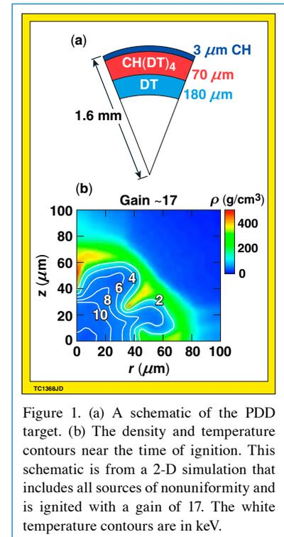
Figure 1. (a) A schematic of the PDD target. (b) The density and temperature contours near the time of ignition. This schematic is from a 2-D simulation that includes all sources of nonuniformity and is ignited with a gain of 17. The white temperature contours are in keV.
