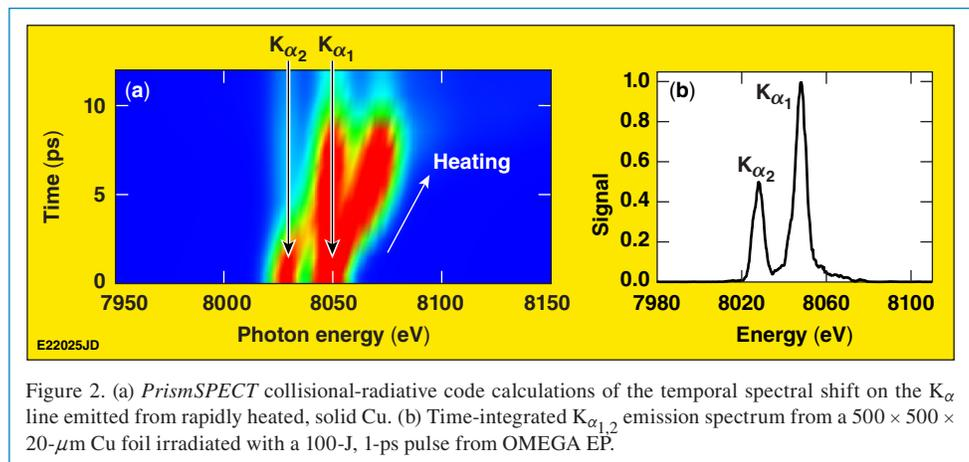
Figure 2. (a) *PrismSPECT* collisional-radiative code calculations of the temporal spectral shift on the  $K_{\alpha}$  line emitted from rapidly heated, solid Cu. (b) Time-integrated  $K_{\alpha_{1,2}}$  emission spectrum from a  $500 \times 500 \times 20\text{-}\mu\text{m}$  Cu foil irradiated with a 100-J, 1-ps pulse from OMEGA EP.
