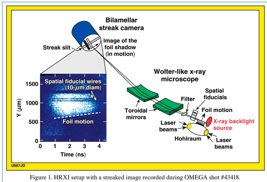
Figure 1. HRXI setup with a streaked image recorded during OMEGA shot #43418.
