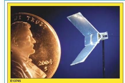
Figure 2. An XRTS target (right) compared in size to a penny.
