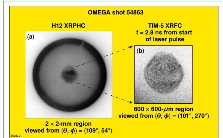
Figure 3. (a) Time-integrated x-ray pinhole camera (XRPHC) image (2 to 7 keV) of polar-drive implosion. (b) Time-gated x-ray framing camera (XRFC) image of implosion core taken near stagnation ( $t = 2.8$  ns from start of laser pulse). In these images, the polar axis is vertical.
