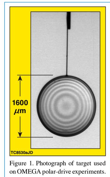
Figure 1. Photograph of target used on OMEGA polar-drive experiments.
