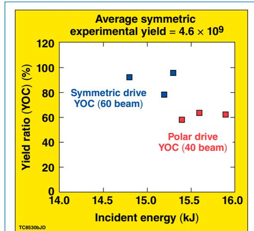
Figure 2. Ratio of measured neutron yield to calculated clean 1-D yield (YOC) (in %) for symmetric implosions (60 beams, blue squares) and polar-drive (40 beams, red squares) implosions at nearly equal laser energy (~15.4±0.7 kJ).
